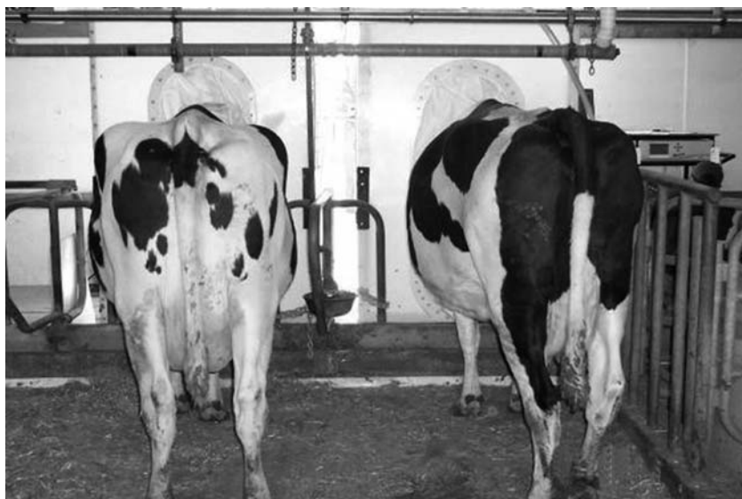
Fig. 10.1. Cows in the ventilated head-hoods during measurement of gaseous exchange (standing).
