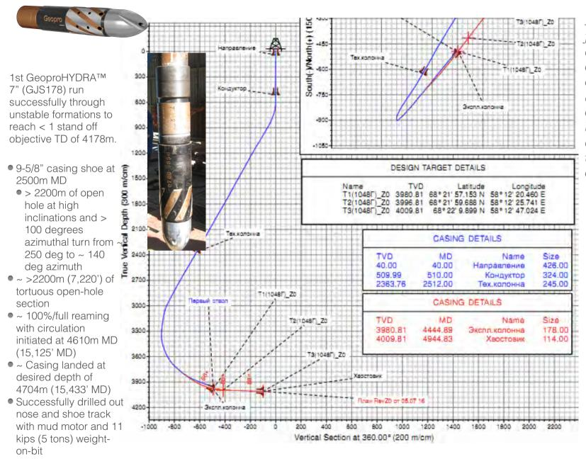
Previous well in the field resulted in 35 days NPT, requiring customer to pull 4000m of 7" casing from well. Severe wellborn conditions prevented landing string at desired depth due to unstable formations and tight spots.
