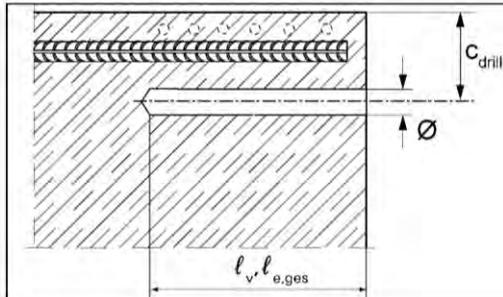
Measure and control concrete cover  $c$
