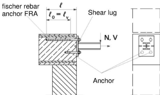
**Figure A8:** Lap of the anchoring of cantilevered building components.
