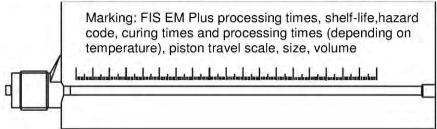
Marking: FIS EM Plus processing times, shelf-life, hazard code, curing times and processing times (depending on temperature), piston travel scale, size, volume
