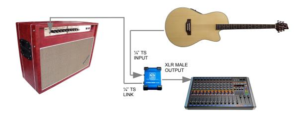
Typical DI Box Setup Diagram
