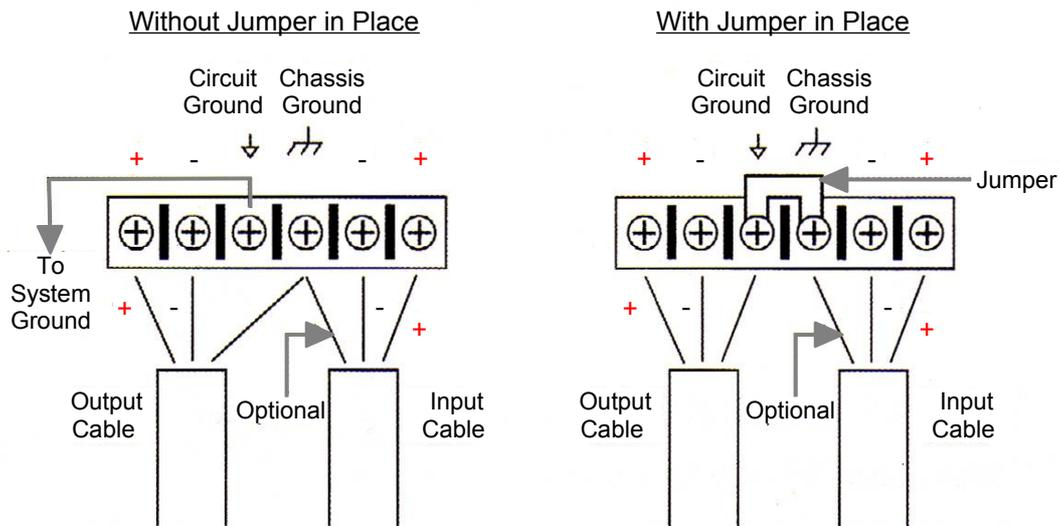
Wiring connectors with ground.
