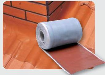
Material: **Articulate aluminium mesh between two layers of polyisobutylene and finished with a waterproofed lining. It has 2 strips of butyl adhesive on the rear.**
