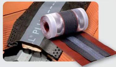
Material: **Lateral laps made from mouldable aluminium and deformable up to 50%, containing water-repellent polypropylene in its central area and a double ventilation channel with a system of geometric openings for optimized ventilation (150 cm<sup>2</sup>/ml) while providing total protection against outdoor elements.**
