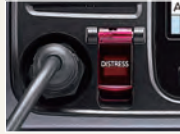
Distress button with a spring-loaded cover
