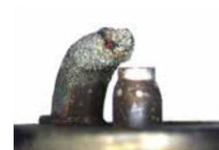
A melted ground electrode indicates pre-ignition. Ensure proper heat range of the plug is used and check ignition timing.
