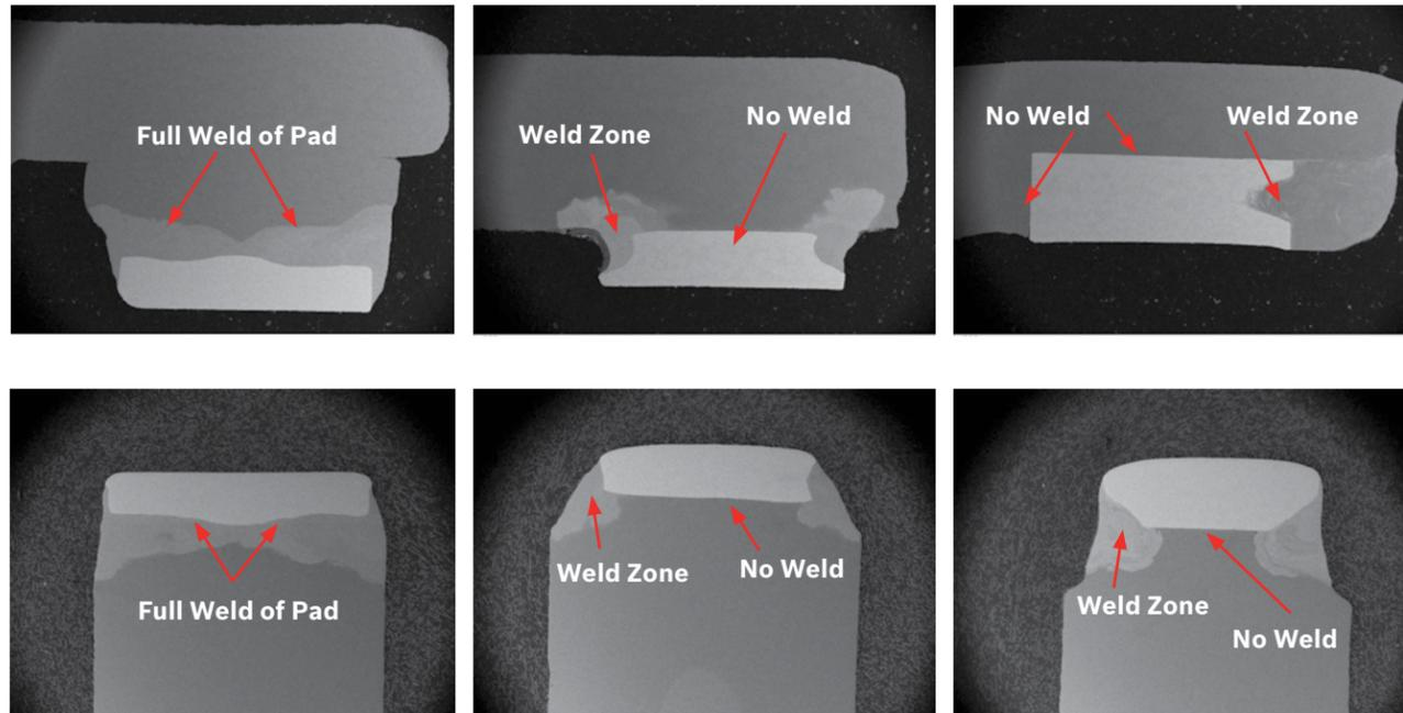
In these cross sections of the electrodes, note that the welding of the Bosch spark plug supports the entire iridium pad. In the other plugs, the welded zone is only on the edges of the precious metal pins. This complete weld, ensures the precious metal pin has the strongest connection possible to the base material and will not separate even in the most demanding applications.
