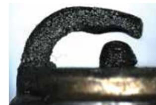
Plugs are coated with oil indicating high oil consumption. This could lead to a spark plug failure such as cracked insulator or oil fouling resulting in difficulty starting.
