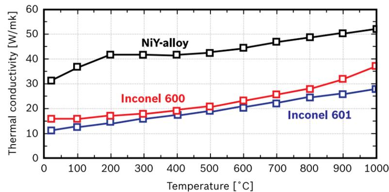
The Nickel Yttrium (NiY) alloy used on the ground electrode of the Bosch Industrial Series spark plugs dissipates heat much better than competitor materials. This results in lower temperatures of the ground electrode and longer run times.
