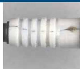
**Flashover:** Spark is traveling over ceramic from the terminal stud to the housing. Check insulator boots for proper fit and replace if necessary
