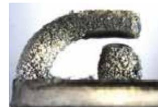
Plugs are covered with normal oil ash. Engine is operating as desired.
