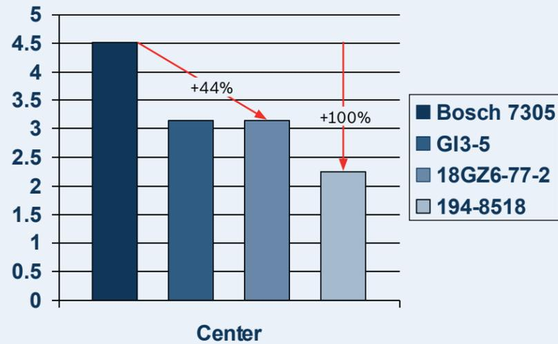
The larger surface area of the center electrode helps increase longevity. The increased precious metal available reduces gap expansion resulting in longer run times.
