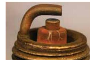
The red coating is iron. The conductive iron leads to misfires as the spark travels from the center electrode to the housing instead of jumping between the electrodes (note white lines on the ceramic). The engine is not operating as desired. Valves may not be seating correctly.
