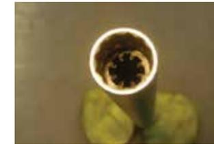
During installation and removal, if the socket is not fully seated on the plug or is applied at an angle, the side force can cause cracks in the ceramic between the housing and insulator.
