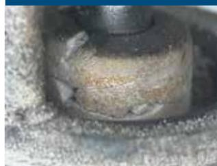
**Ceramic Puncture:** Punctures in the ceramic caused by high ignition voltages
