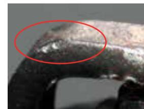
Plug was damaged during installation or impacted during use. Use caution when installing new plugs. Do not drop plugs into cylinder head during installation.
