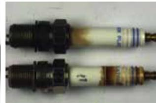
M18 plugs should be torqued to 35-45 Nm (26-33 Lb-ft)
