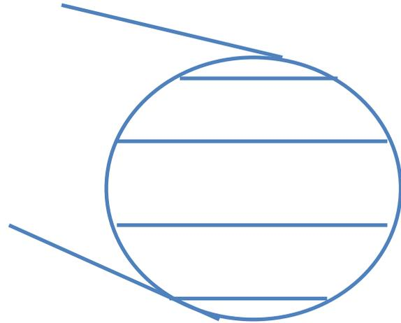
Consequently, ultrasonic meters generally measure the velocity at multiple horizontal points in the pipe, with each called a path, and as such the meter is multipath.
