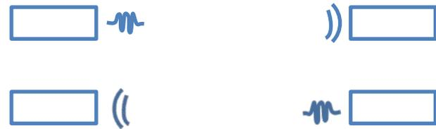
Each path has a transducer pair, which is generally piezo-electric, which when a voltage is applied makes a sound wave, and when it receives a sound it creates a small
