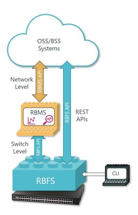
RtBrick's REST APIs are based on a Model View Controller (MVC) design, so nothing is masked from the operator. There is no intermediate layer, so you have access to every feature that you can control with a traditional CLI (Command Line Interface).
