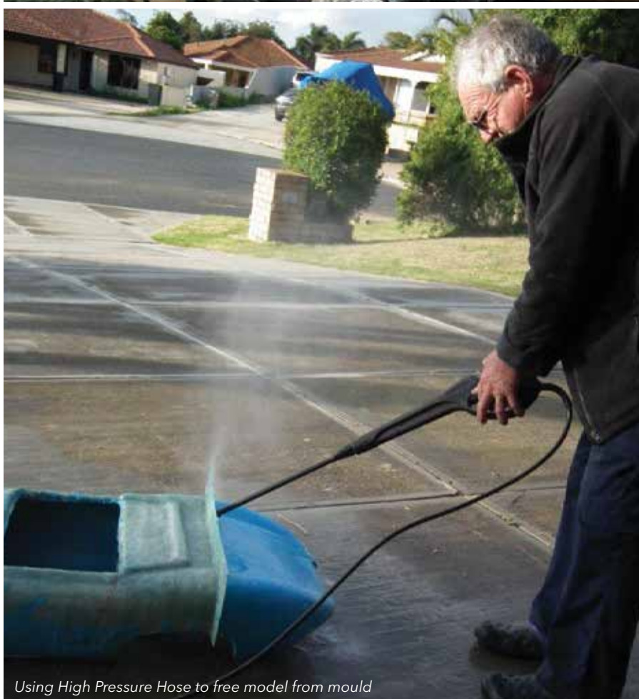
Glass fibre mould on polystyrene buck
