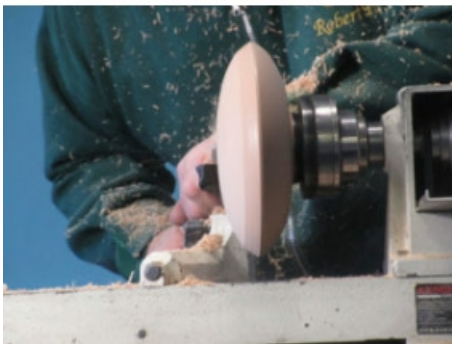
This picture shows the shape Robert wanted and he sands it to a very good finish as any imperfections will show up worse by the finishes.
