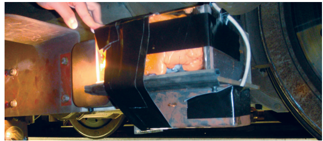
Figure 5: Back view of the camera assembly with tape that protects the video and sync from coming out of the rear
