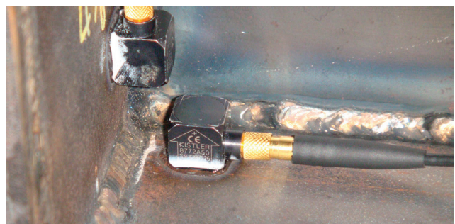
Figure 8: Accelerometers glued to a rigid plate
