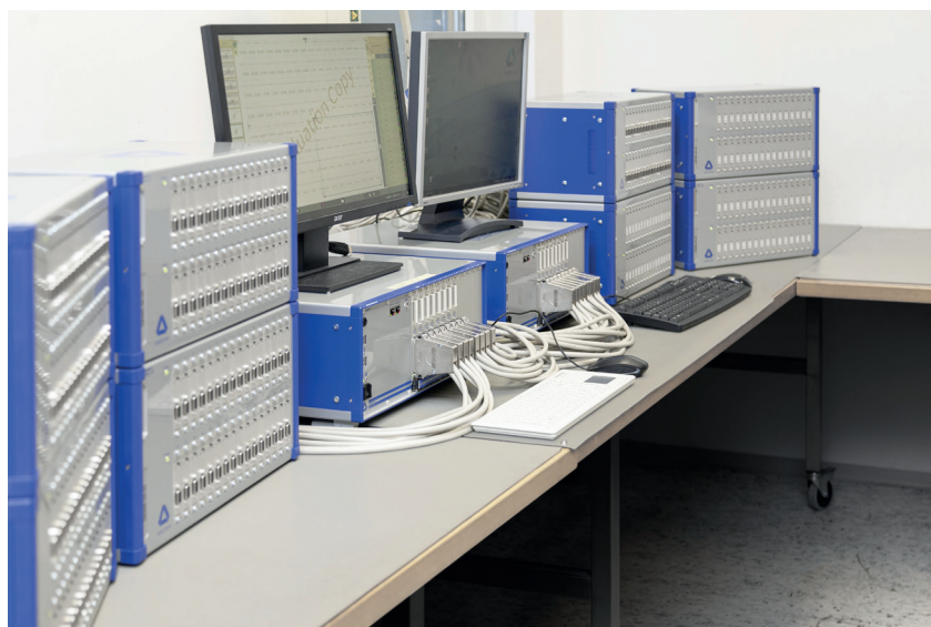
Figure 5: Signal Conditioning and DAQ system during quality check (Desktop PCs not included)
