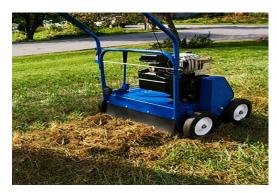
There are several names for effective dethatching equipment: vertical mowers, verticutters, dethatchers or power rakes.
