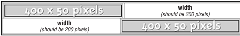
Figure 10-16: Since the middle column was not defined, the table is rendered with two 400-pixel-wide columns
