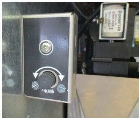
Fig.39 - Milk foam adjustment
