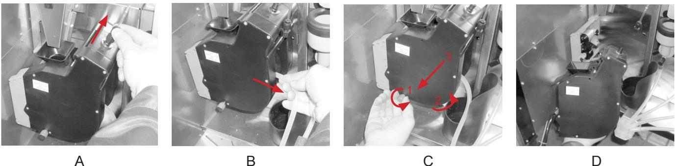
Figure 26 - Removing the espresso group
