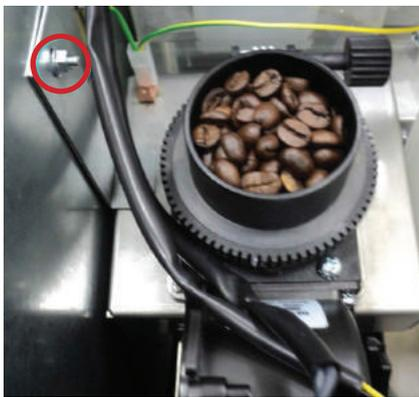
Figure 2 - Removal of the transportation bracket
