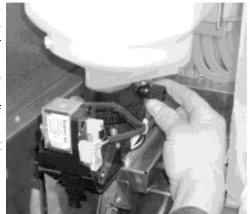
Figure 22 - Adjustment of grinding
