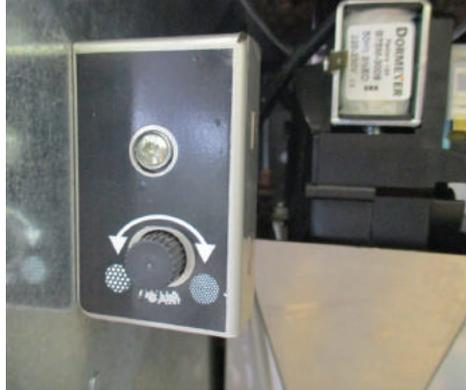
Fig.41 - Milk foam adjustment
