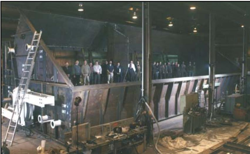
SCR Diverter (9 foot 6 inch wide by 66 foot 10 inch flap) with more than 20 workers standing on the flap. This diverter was later shipped and placed into service in the United States
