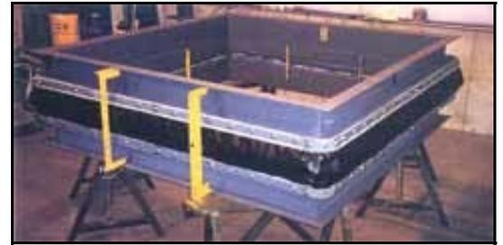
8 foot square boiler flue gas expansion joint. 20 in wc at 800°F.
