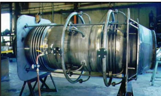
Pressure Testing of Bachmann Metal Expansion Joint
