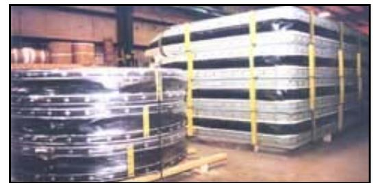
Various non-metallic expansion joints for boiler flue gas application awaiting shipment.
